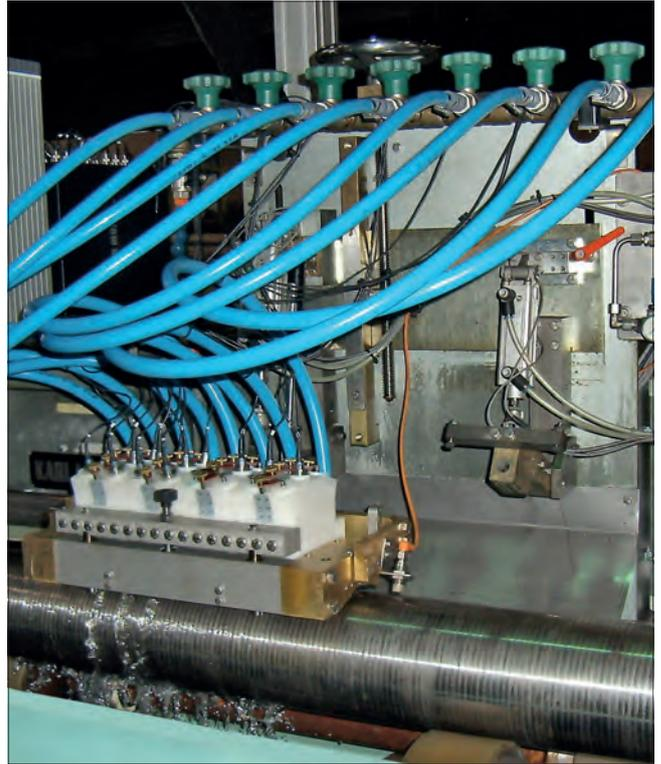
Testing portal for steel bars with one common probe holder. In this case 8 straight beam probes and 16 angle beam probes (8 clockwise, 8 counter-clockwise) are used. This results in a test track of 80 mm per revolution.
