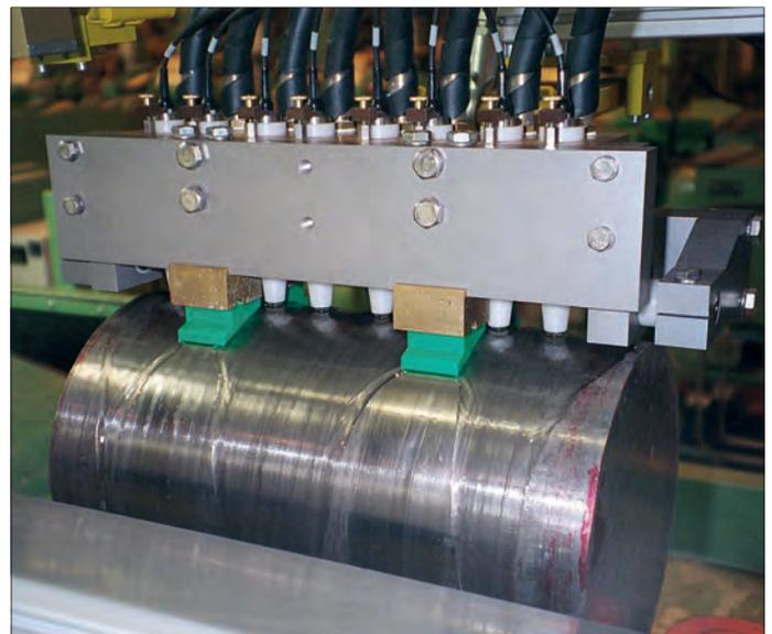
Closer view of a common probe holder with eight straight beam probes. A (white) water nozzle guides the ultrasound for each probe. In this case, (green) plastic skids are used to protect the machined billet surface.
