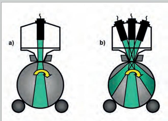
The distance between ultrasonic probe and billet is kept constant by guiding the probe holders along the billet surface by means of skids and/or rollers. The straightness deviations require a gimble joint for the probe holders to perfectly follow the billet surface.
