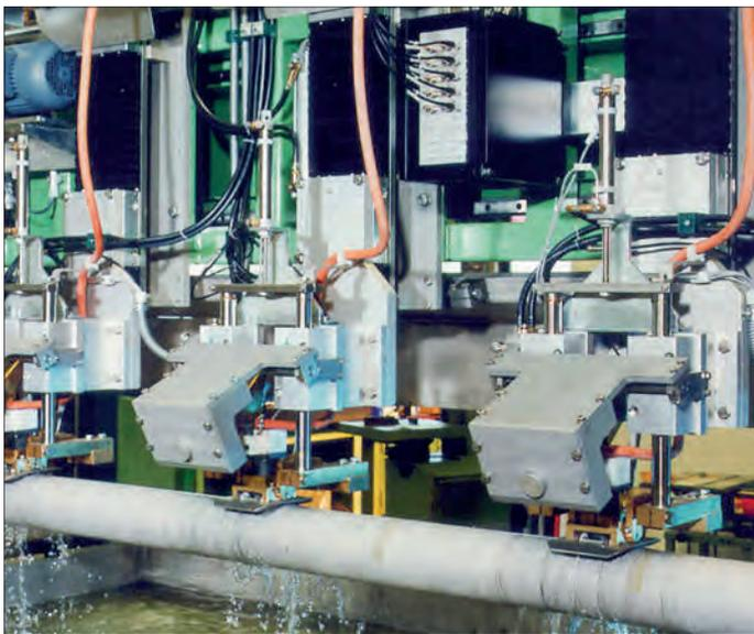
Here, each probe holder contains one straight beam probe. A large metal skid protects the probe and the water nozzle from damage. The cast surface of this aluminium billet is quite rough.
