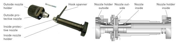
Fig. 15: Protective nozzle and nozzle holder standard
