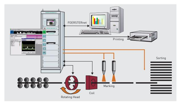
Fig. 1: Application CIRCOGRAPH with DEFECTOMAT channel for piece testing
