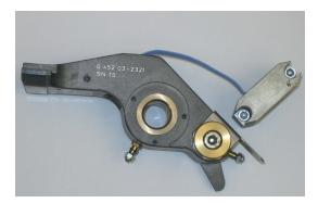
Fig. 9: Test head in lever design
