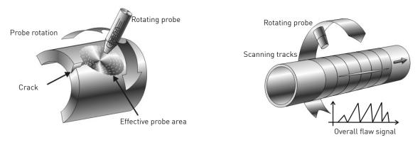
Fig. 2: Rotating probe at material defect
