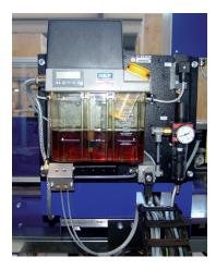
Fig. 19: Oil Air Lubrication
