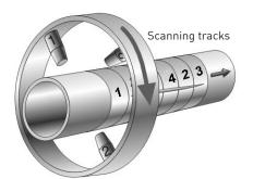
Abb. 4: Scanning tracks with four probes (90° offset)
