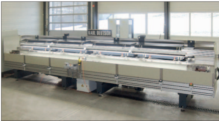
This HW testing system with direct current magnetization for steel bar testing allows rotation and visual evaluation directly in the system.
