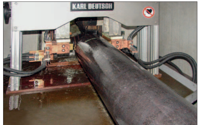
Seamless tubes can be linearly fed through a combination of magnetizing yoke pair and coil.
