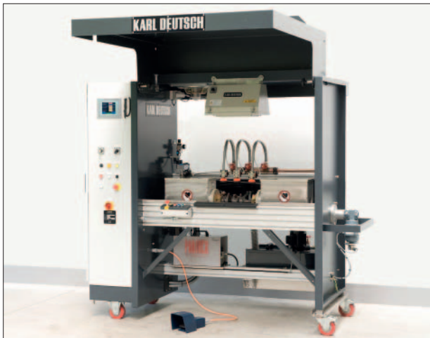
The UWE 350 testing system provides clamping lengths of up to 350 mm. This example shows a mobile test bench with a motorized adjustment of the clamping length, MEMORY PLC software, heavy duty rollers and a folding roof – perfect for service inspection companies.
