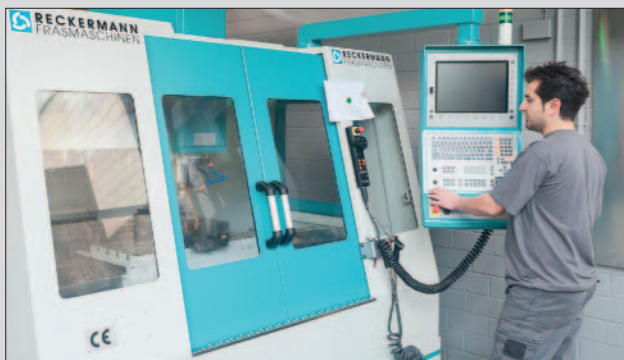
Modern machinery is used for the in-house production of mechanical parts. The picture shows a CNC-machine which is able to import CAD-data for fast processing and production.
