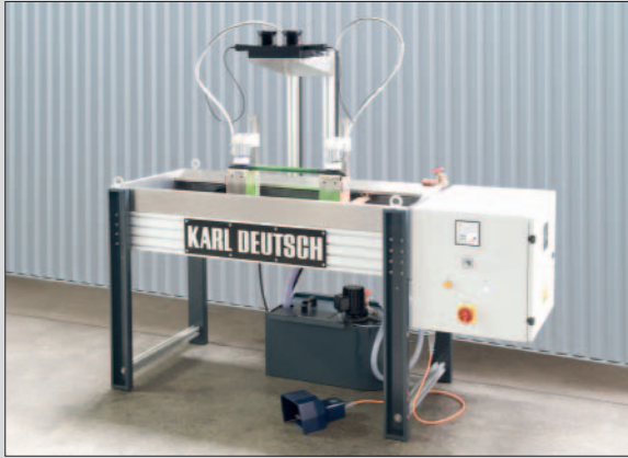
The HW testing system provides a circular magnetization produced by a direct current flow for the detection of longitudinal cracks (e.g. for wire testing). The system contains a fixture for two mobile UV-LED lamps which can be easily removed for flexible evaluation of all test piece surfaces.
