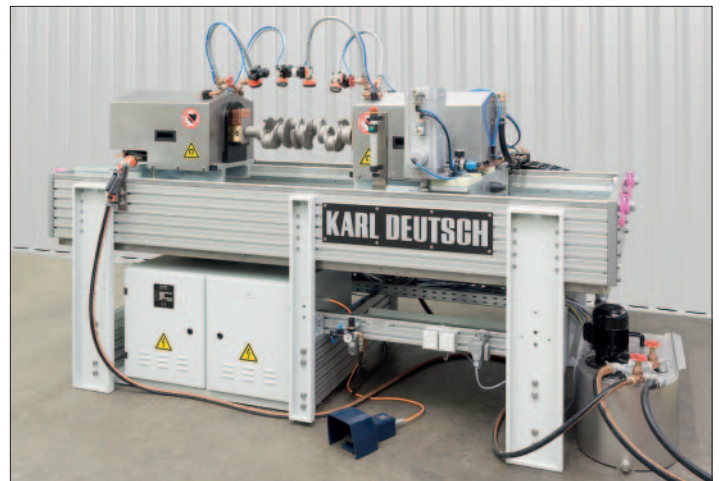
This example shows a special version of a UWE bench with a test mechanic of low height for convenient loading. It is therefore well suited for production lines with a high level of automation. The adjustment of the clamping length can be motorized and automated.
