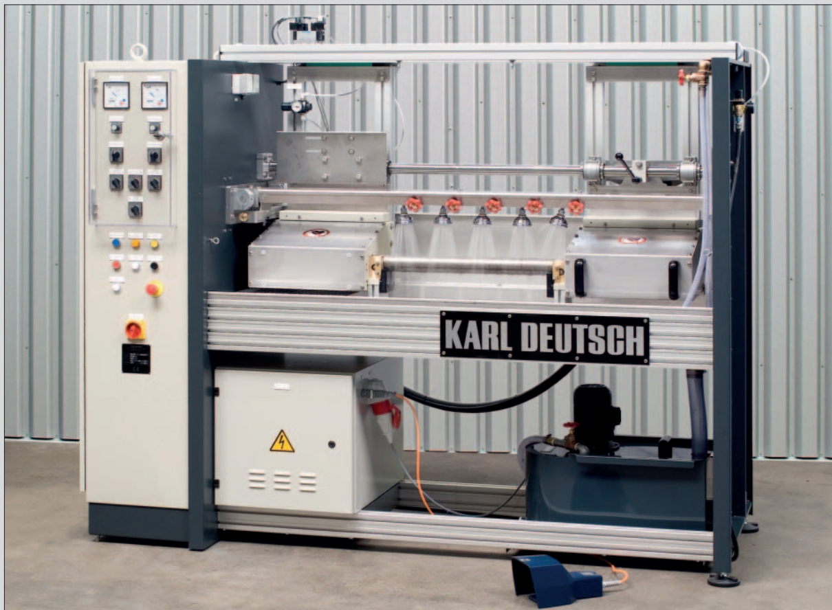
DEUTROFLUX UWE: Universal test bench with two contacts and multi-directional magnetization. Both fields can be adjusted independently. The test bench is available in three sizes. The maximum length of the test piece is then 350 mm, 600 mm or 900 mm, respectively. A release handle for the adjustment of the clamping length is mounted outside the spraying area. Therefore, a smooth-running adjustment is ensured. The picture shows a pneumatic spraying unit which automatically moves backwards after the designated spraying time.
