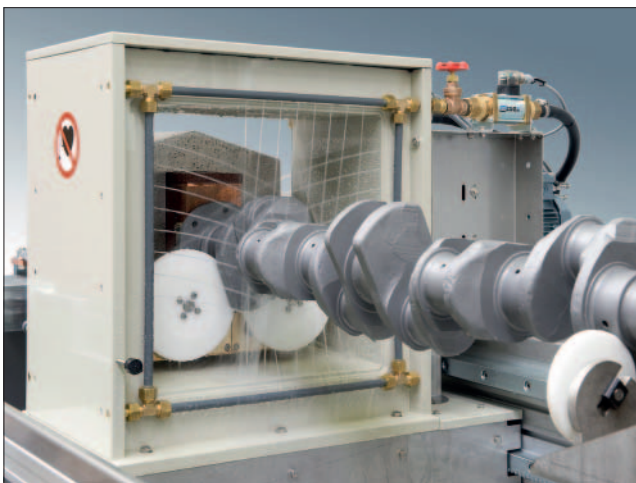
Moving coil with ring of nozzles for crankshaft testing
