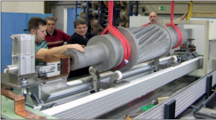
The inspection of a large pinion shaft with a weight of 4 tons is carried out by means of a specially designed moving coil.
