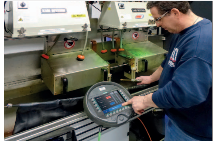
As needed, mobile touch panels are provided.
