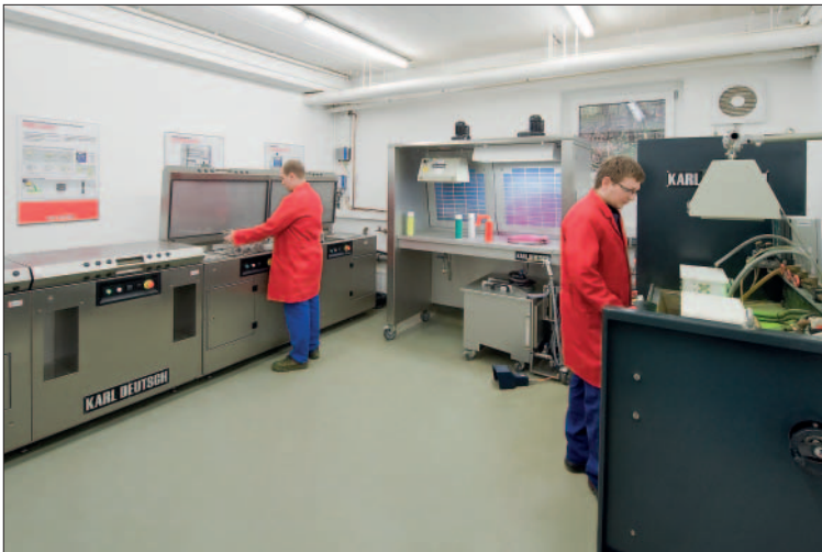
Three application laboratories in both workshops are available for customer-specific trials. The available equipment also includes fully operational MT and PT systems. Test method and magnetic ink can be optimized for the samples handed in by our customers.
