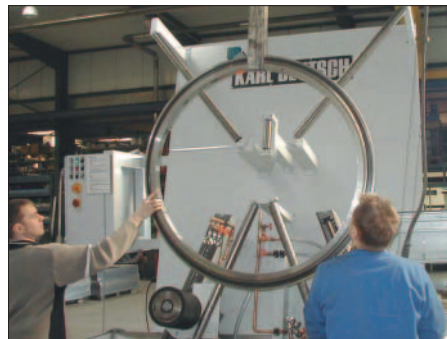
Large rings for wind turbines are often tested in vertical position. The inspection requires one full rotation.
